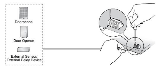
2. Attach the terminal blocks to the connectors of the DPH4/DPH2/EIO4 card on the Hybrid IP-PBX.
