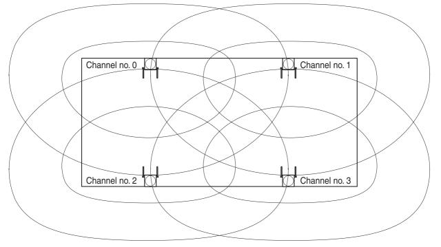
**c.** Make sure that the radio signal strength level is greater than "3" at any location in the service area demanded by the user.
