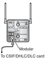
2. Pass the cable through the groove of the CS (in any direction depending on your preference).
