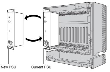
5. Follow the steps in "Installing the Power Supply Unit".
