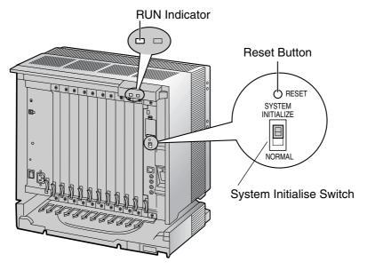
2. Plug the AC power cord into the Hybrid IP-PBX and an AC outlet, and turn on the Hybrid IP-PBX. The RUN indicator will flash.
