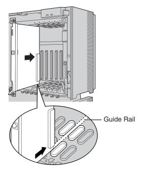
2. Holding the card as shown below, push the release lever in the direction of the arrow so that the card engages securely with the connector on the back board.
