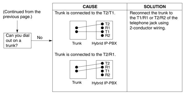
Connection between the trunk and the Hybrid IP-PBX:
