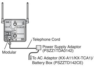
**4.** Install the CS temporarily for the site survey. Install the CS at least 2 m above the floor, keeping the antennas in the upright position.
