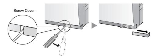
2. Turn the screw anticlockwise to loosen.
