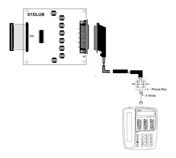
Figure 21. Digital Key Station Wiring on D1DLUB
