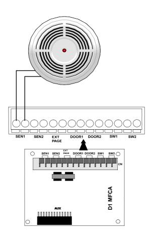
Figure 25. External Sensor Wiring on D1MFCA
