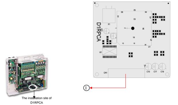
Figure 14. D1RPCA (Remote Programming Card)
