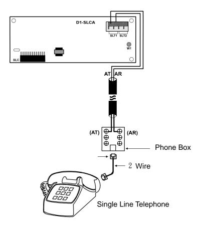
Figure 23. SLT Station Wiring on D1SLCB
