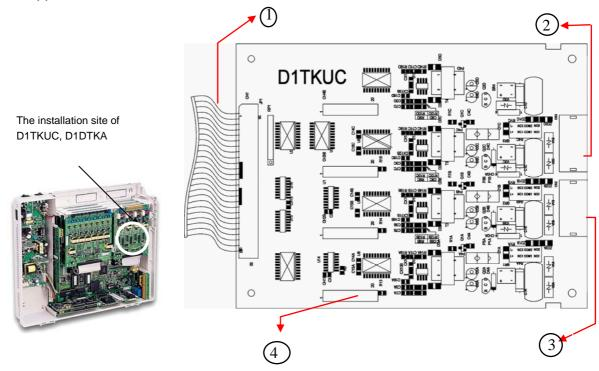
Figure 4. D1TKUC (TRUNK UNIT, 4 TRUNK PORTS)
