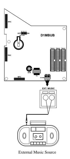
Figure 27. External Music Source Wiring on D1MBUB
