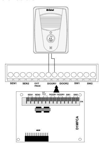
Figure 24. Door Phone Wiring on D1MFCA
