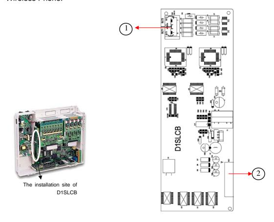
Figure 8. D1SLCB (Single Line Station Card, 2 SLT Station Ports)
