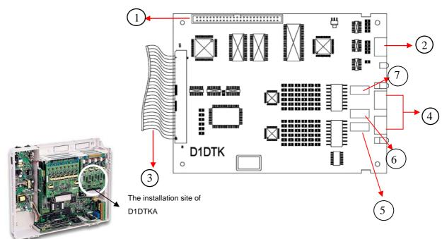
Figure 5. D1DTKA (ISDN TRUNK UNIT, 2 BRI PORTS)
