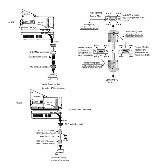
Figure 28. RS232 Wiring on D1MBUB (wired by customer)
