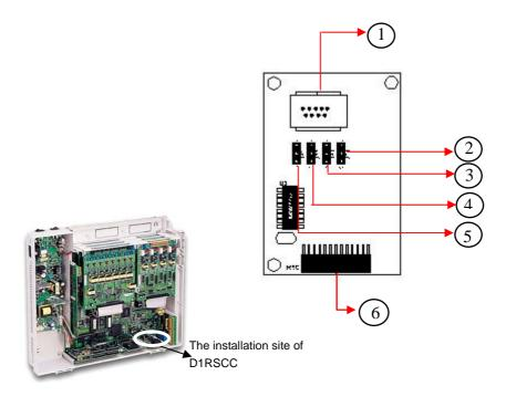
Figure 9. D1RSCC (RS232 Card, 2400bps Serial RS232 Port)
