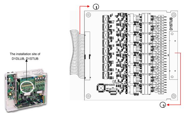
Figure 7. D1STUB (Analog Key Station Unit, 8 Key Station ports)
