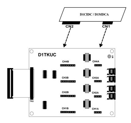
Figure 20. Metering Pulse Detection Card Installation
