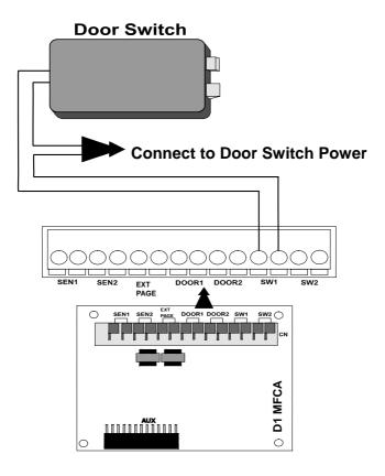
Figure 26. Door Switch Wiring on D1MFCA
