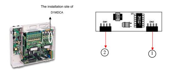
Figure 12. D1MDCA (Metering Pulse Card)
