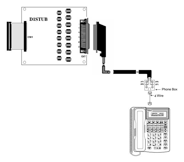
Figure 22. Analogy Key Station Wiring on D1STUB
