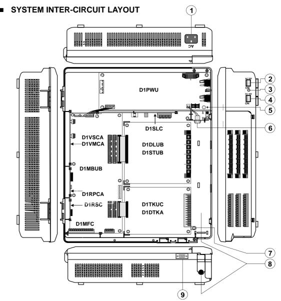
Figure 1. System Inter-Circuit Layout
