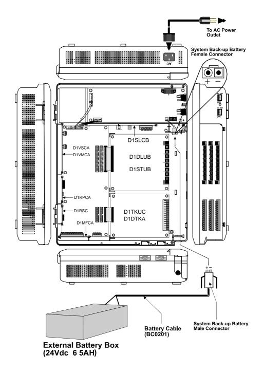
Figure 18. AC Power and DC Battery Back-Up Installation
